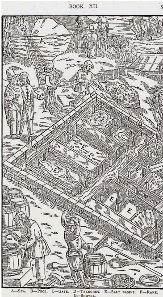
Fig. 2. Sixteenth century salt making from seawater. (Agricola, 1950 trans.)
