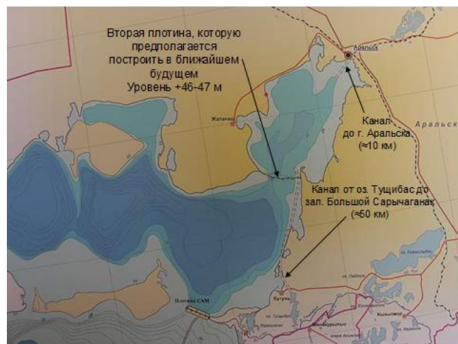
Figure 14: Possible location for the new dam
